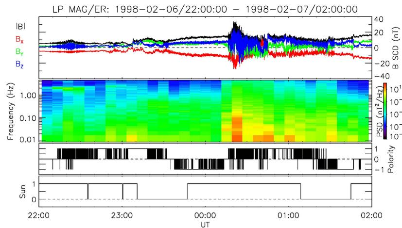
**Figure 1:** Lunar Prospector (LP) magnetometer data during a bow shock crossing. Top to bottom: magnetic field, FFT of 9 Hz magnetic field data, magnetic connectivity flag, and Sun flag.
