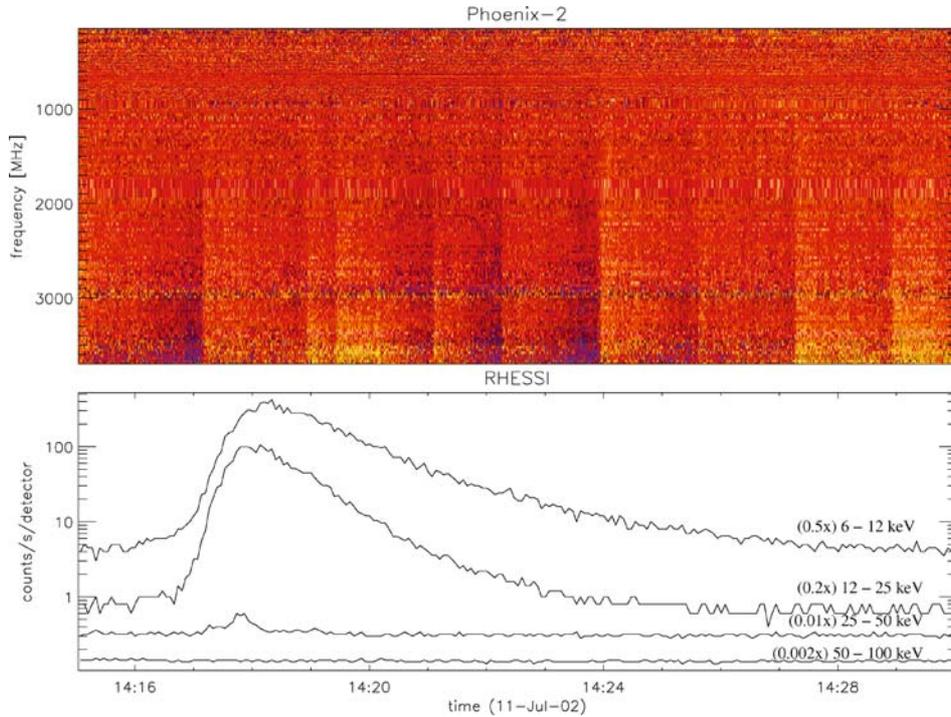
Figure 9. The light curves of an M1.0-class flare. Soft and hard X-ray emission is observed by RHESSI, but no radio bursts in the 0.1–4 GHz band surveyed by *Phoenix-2*.
